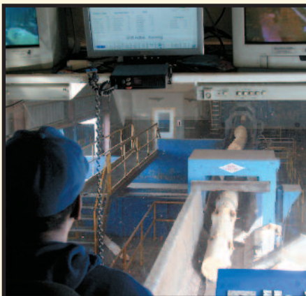
Willie Alderman in control cab overlooking MDI metal detectors on primary line
